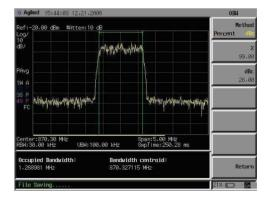
The occupied bandwidth is measured in dBc.
